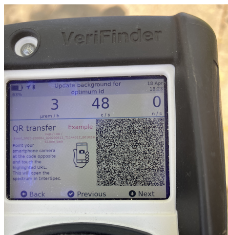
Figure 0-5. Example images captured of the Symetrica Verifinder displaying a QR code. This screen is displaying a ‘canned’ QR code that was pre-generated. The handful of tested QR codes could be reliably read in with a phone, both indoors and outdoors.
