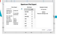
Export the spectrum as a N42-2012 file. This will save all fit peaks, nuclide IDs, Energy calibration, detector efficiency function, and your Activity/Shielding fit, into a N42 file
